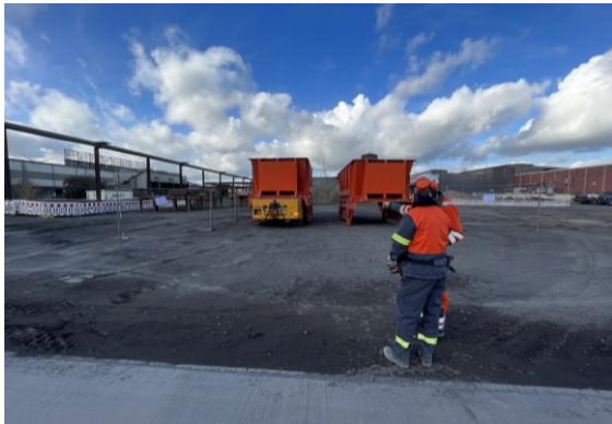
Hot boxes at a cooling location. One box is put down to cool, while another one with solidified slag is being taken to the tipping device.
