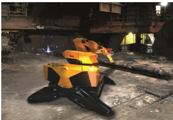
UNIDACHS 110 – Blast furnace runner break out
